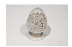
The silica ramming material is pre-mixed dry ramming
